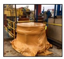
**VAPPRO 826MW VCI MIL-WRAP** is a significant breakthrough in protective packaging technology. It offers a new concept in corrosion protection without the need for oily rust preventative coatings.
