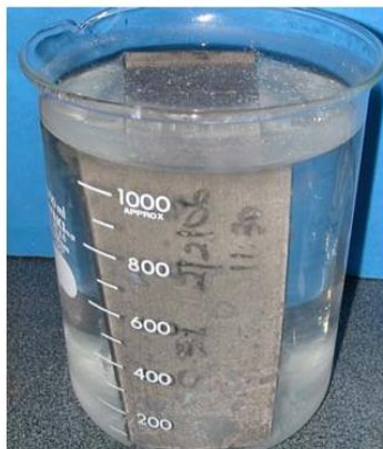
Mild steel immersed in sea water with 0.05% of Vapro 844
