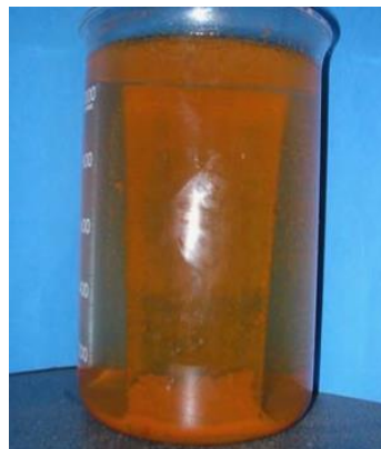
Mild steel immersed in sea water without Vapro 844
