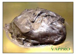
**VAPPRO 999** is a metallic silver high temperature grease made from a high VI olefinic copolymer and a finely divided thickener. This grease is fortified with VCI additives that provide it with excellent lubricating properties, stability and anti-wear capabilities.
