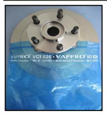
**VAPPRO 9874** is a solvent-based liquid VCI corrosion inhibitor. It is specifically designed for the corrosion protection of metal parts such as brake rotors during cryogenic test cycles. After the solvent evaporates the residual micro-film formation is highly resistant to corrosion.
