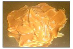
**VAPPRO 869** is a mixture of vapour corrosion inhibitors and oilbased carriers. It is formulated to provide superior protection over conventional rust inhibiting oils and coatings. **VAPPRO 869** concentrate is a grease-like material that is diluted with oil to provide a self-healing lubricating coating. **VAPPRO 869** can also be added to lubricating oils to improve corrosion resistance.
