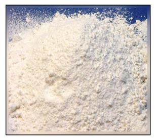
**VAPPRO 841** is an odourless VCI powder specially developed to inhibit both ferrous and non-ferrous metals from corrosion after hydro-testing. It eliminates the formation of corrosion due to residual water after draining hydro-test water.
