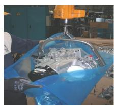
**VAPPRO 826 VCI Film** is a significant breakthrough in protective packaging technology. It offers an innovative concept in corrosion protection eliminating the need for rust preventative coatings.
