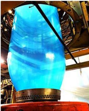
The let-down ratio of **VAPPRO 1000 MBR** is **6% by weight**. By means of a rotating mixer, mix the VCI Masterbatch Additive thoroughly with virgin PE resins prior to extrusion.
