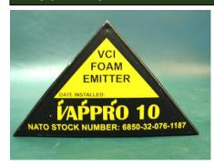
**VAPPRO 10 Foam Emitter** is a triangular foam pad impregnated with vapour corrosion inhibitors. This VCI foam emitter is particularly suitable for corrosion protection in enclosures holding electrical gears, relays, contactors, switches, electronic assemblies and connectors. The vapours do not increase contact resistance in relays and switches and will not affect the characteristics of insulating materials which include high voltage corona or carbon tracking.
