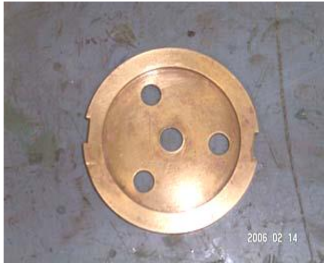
Aerospace brass plates protected with V-9600
