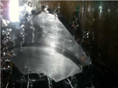
Gray iron treated with V-853 inside 100% Humidity Chamber
