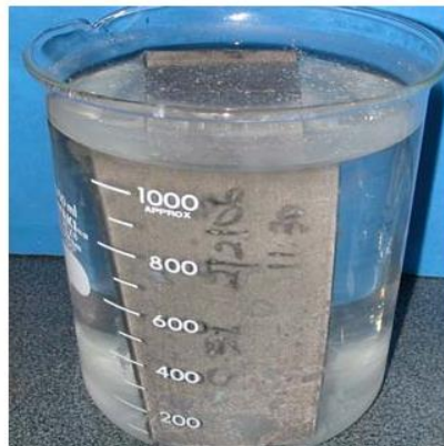
Mild steel immersed in sea water with 0.05% of Vapro 844
