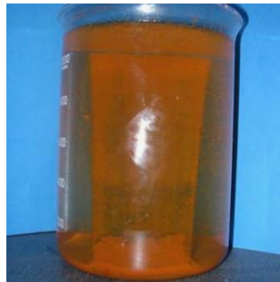
Mild steel immersed in sea water without Vapro 844
